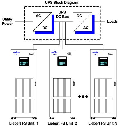
Figure 3 Liebert FS unit(s) integrated into UPS system for ride-through to backup generator UPS Block Diagram
